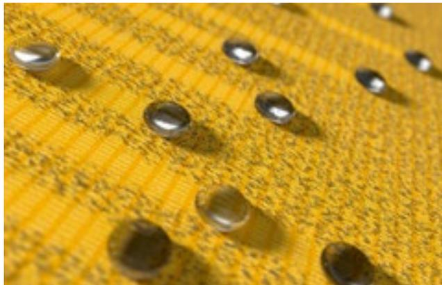
**Self-cleaning snc effect** Water droplets pick up dirt particles and run off the awning cover (the awning must be set at a pitch of at least 14 degrees). This gives you the peace of mind that your fabric will retain its colour and vibrancy for years without you having to lift a finger.
